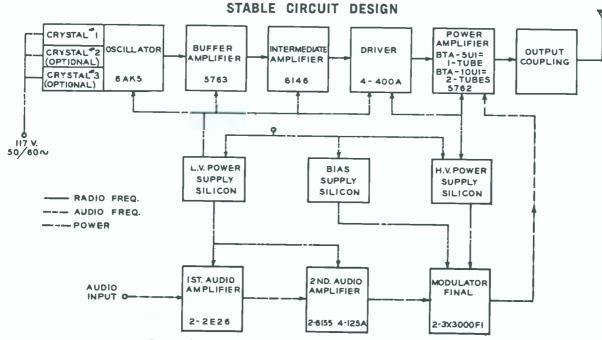
Block diagram of Type BTA-5U1 and BTA-10U1 Transmitters.
