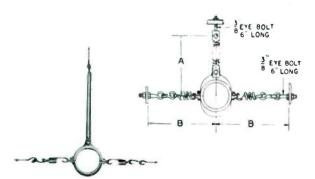
Spring hanger for horizontal suspension of single line. Anchored at three points. Complete with eye bolts and springs.
