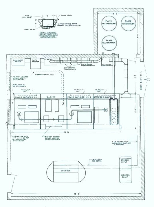
Typical floor plan for the BTA-50H1 Transmitter.
