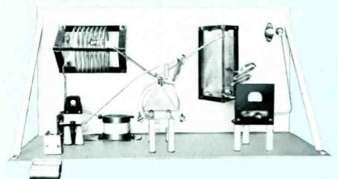
Line Terminating Unit installed on open panel.
