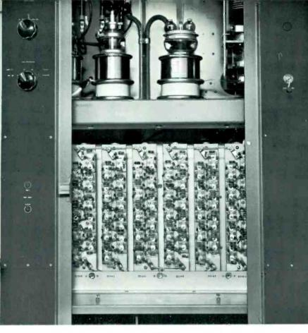
Front view of the Silicon Rectifier Chassis of the BTA-5T1. The silicon cells offer improved performance since they are particularly resistant to aging, moisture and wide temperature variations.
