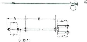
Maintains single line at fixed distance from tower or building. Mounts through single hole. Complete with two clamps.
