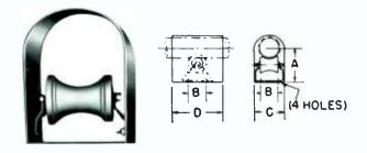
Supports single line. Roller permits line expansion. Hood protects roller. Mounting bolts not supplied.
